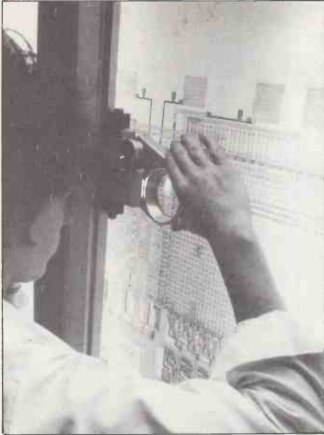
Checking one of the many masks, drawn several 100 times final size.
